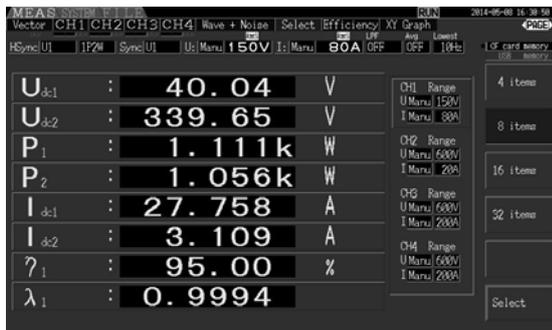
Fig. 7. An example of the operating point of the converter
