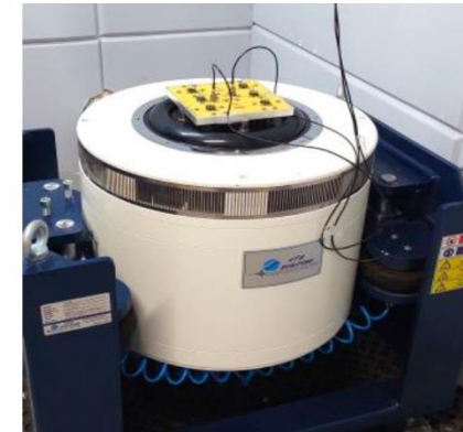
Pic. 10 Z-Axis Vibration Test
